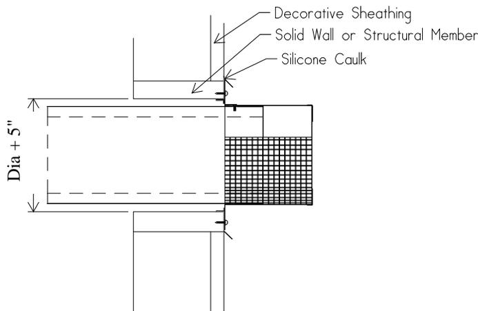
may be reduced if necessary. If there are not sufficient support members to secure the Wall Penetration Assembly or if there is a semirigid foam insulation layer under the sheathing, the opening must be blocked out or framed to provide support.
